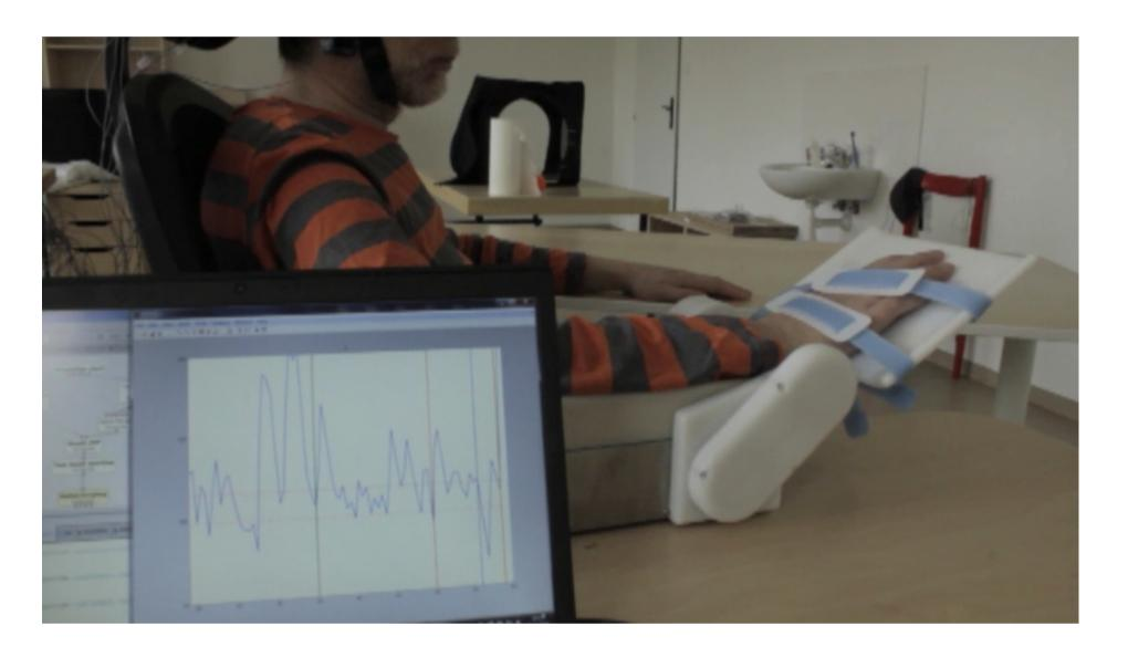
To vary the difficulty of controlling the robotic splint, a set of different training protocols and time-scores threshold levels are investigated. Figure below shows the numbers of successful moves (out of 10 trials) of the splint (i.e. successful  $\mu$ -rhythm desynchronization during motor imagery, manifested by getting under the preset power threshold, compared to relax state).
