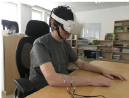
Figure 3: A picture of a subject with Oculus Quest 2 head-mounted display, g.tec g.Nautilus Pro wearable EEG headset, and functional electrical stimulation (FES) electrodes applied to the subject's forearm group of muscles.
